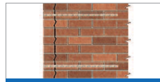
3 Repairing cracks near corners and openings
